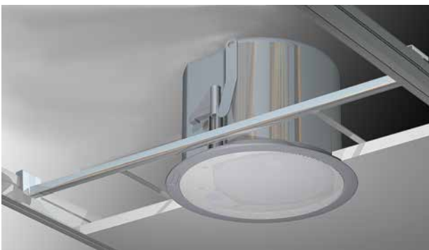
Figure 6. Position of loudspeaker relative to bridge support rails during installation Align the flat sides of the can with the tile support rails
