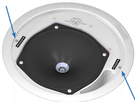
Figure 8. Turning the two loudspeaker clamp actuators clockwise securely locks the unit into the ceiling.
