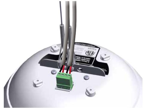
**Figure 5.** Wire and insert second connector for daisy-chain connection to another loudspeaker
